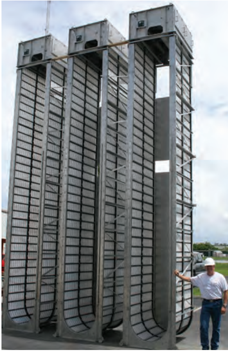
300+ gpm sluice hydraulic capacity test at factory.
