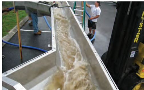
300+ gpm sluice hydraulic capacity test at factory.
